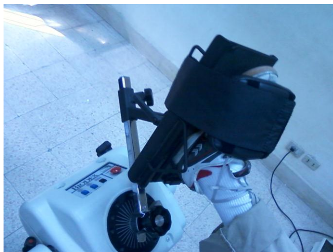
Figure 2. Foot position during measurement of invertors and evertors eccentric peak torque
