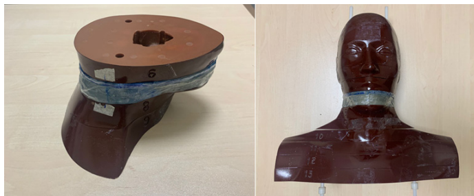
Supplementary Figure S1. Planning CT setup of the Rando phantom with epoxy-BaSO 4 bone-equivalent inserts
