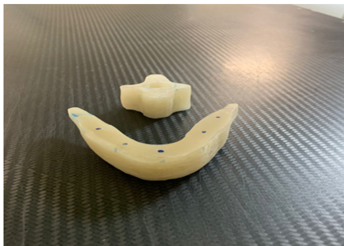
Figure 1. CT images of epoxy- \text{BaSO}_4 composite inserts for the cervical and mandibular regions
