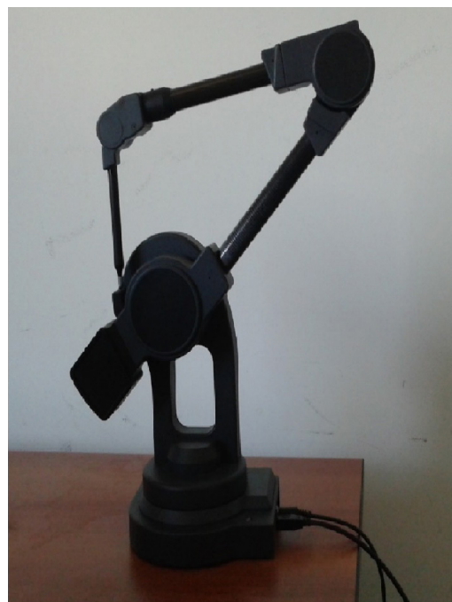
Figure 2. The MicroScribe-Gx device used in measurements
