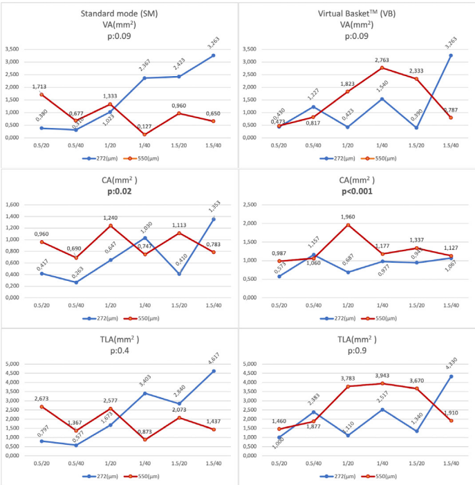
Figure 4. VA (vaporization area), CA (coagulation area) and total laser area (TLA, calculated as VA+CA) values of different laser settings of 272 (μm) and 550 (μm) laser diameters in Ho:YAG laser SM and VB modes
