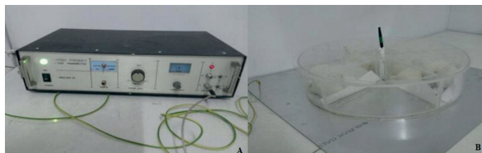
Figure 1A. 1.8 GHz emitter (1800 CW2; Everest, Adapazarı, Türkiye) 1B. RF-EMF exposure application of rats is made in the center of the pie cage restrainer consisting of 5 slices in vertical position
